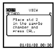
If it is necessary to abort the calibration sequence before all standards have been measured, this can be carried out by pressing any keys other than **CAL** or **ENTER**. Only information entered up to that point will be retained.
