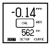
Remove the sample blank from the sample chamber and replace with the unknown sample. The Absorbance value is read and plotted against the curve to determine the concentration value. This value is presented in large figures at the top of the screen.
