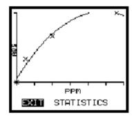
Selecting **STATISTICS** from this menu will show the terms used for the calculated quadratic curve fit. The curve fit is of the form  $y = ax^2+bx+c$ , so the statistics page shows the  $ax^2$ , bx and c terms separately.
