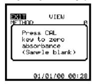
Press the CAL key again with a sample blank present in the sample chamber. The display will momentarily show CAL.
