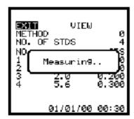
and then update, requesting the next standard to be placed in the sample chamber until the specified number of standards has been calibrated.
