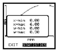
If unlocked it is possible to adjust/amend the standard or Absorbance values by using the right arrow key to move over to Absorbance values.
